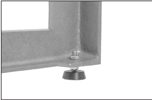
Figure 12. Machine feet installed.
